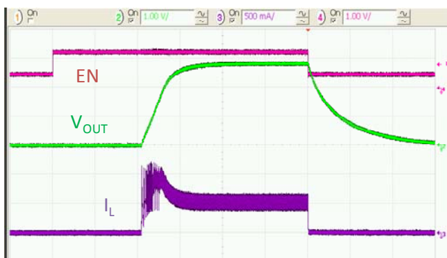
Figure 18. Startup and Shutdown through V_{EN} with 500mA Load, 50μs/div.
